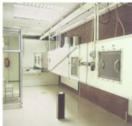
Performance testing in the EN 779 test duct.
