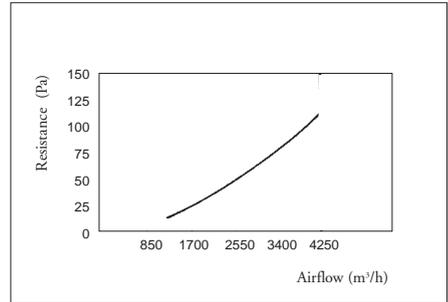
Airflow resistance for a clean 24x24 pad, rated airflow is 3400 m³/h.
