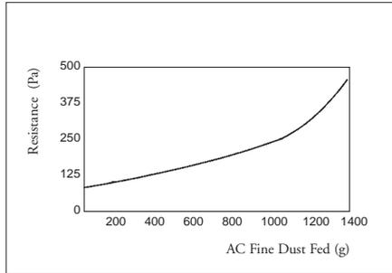
Dust holding capacity for a 24x24 pad with AC fine test dust at rated airflow of 3400 m/s.
