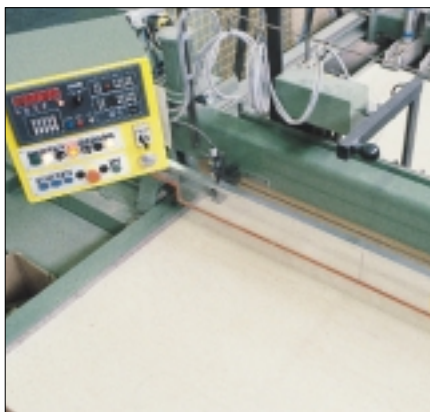
NC saw cutting cell sides
