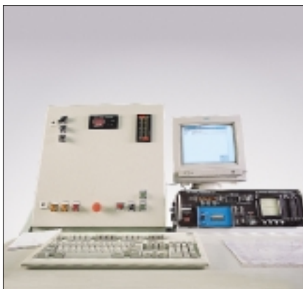
Laser spectrometer efficiency testing control unit
