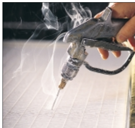
Leak test and pinhole repair (DIN 24.184)
